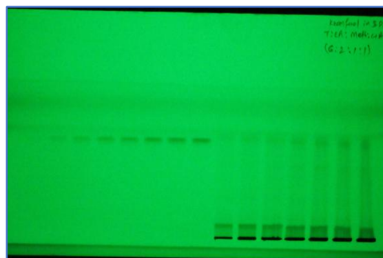
Figure 5: HPTLC Plate Visualised at 254 nm Showing Standard and Sample Bands
